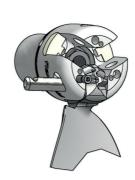
4 Continue with the next two blades; Work blades open and folded to ensure ease of operation; Tighten all pivot pin locking screws using the Allen wrench supplied. If using torque wrench tighten to about 1.2 Kpm = 12 Nm = 8.4 ft-lb.; Again work blades open and folded to ensure ease of operation;
