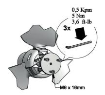
**6** Mount sacrificial anode (11) Zn or AlMg, with one socket-head cap screw (12) after having applied thread locker to threads if not already applied.
